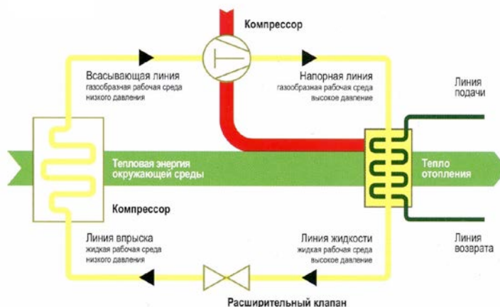
Figure 1. Heat pump's principle of operation [20]
