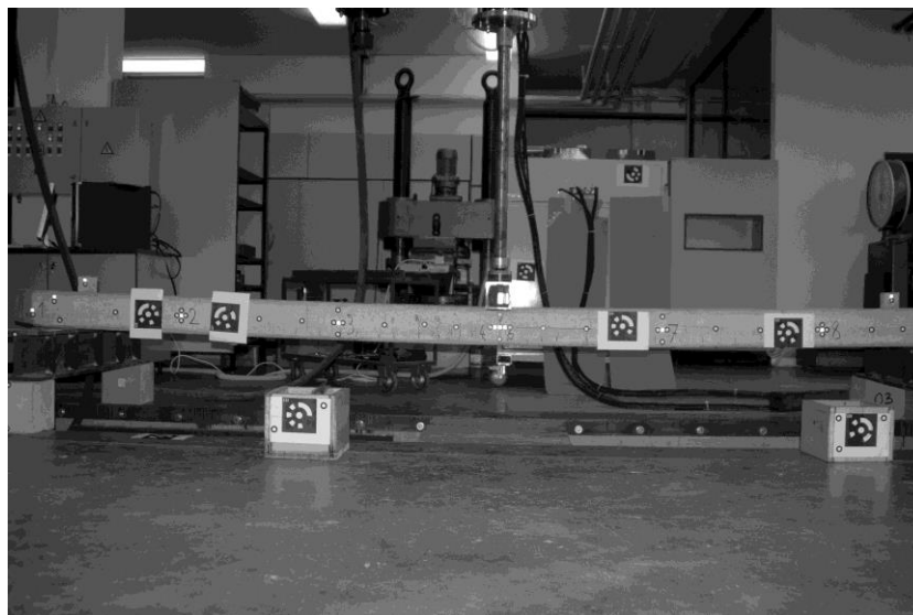
Figure 1. Prefabricated prestressed concrete plate with measured marks
