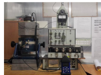
Figure 3. Device for the determination the elacticity modulus
