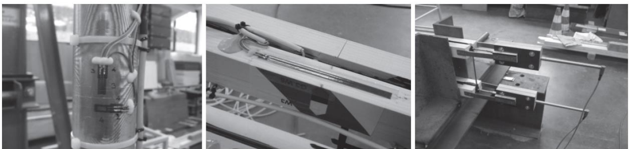
Figure 6. a), b) strain gages on piston and on wood and glass c) inductive displacement sensors at the end of the beam
