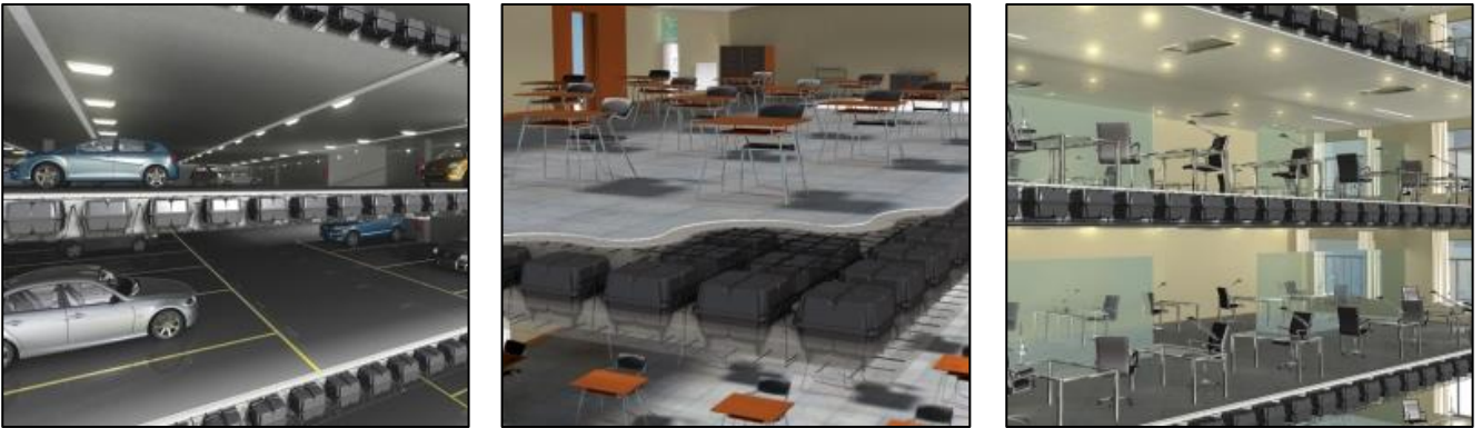
Figures 5-7. U-boot® slab application [7]
