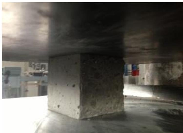
Figure 2. Strength tests on the concrete sample, after a period of care
