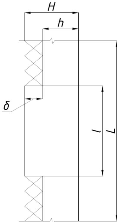
**Figure 2. Analytical model of enclosing substructure**
