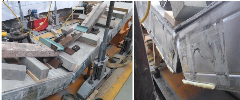
Figure 5 – LSCS - slab panel behaviour crush
