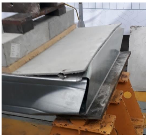
Figure 7 – LGSS - slab panel behavior crush (case of collapse on the support)
