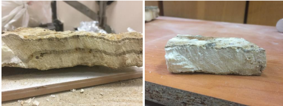
Figure 2. The resin samples, extracted from the injection site after the injection process of the field experiment.
