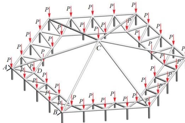
Fig. 1- Coating structure under uniform load  $n=4$
