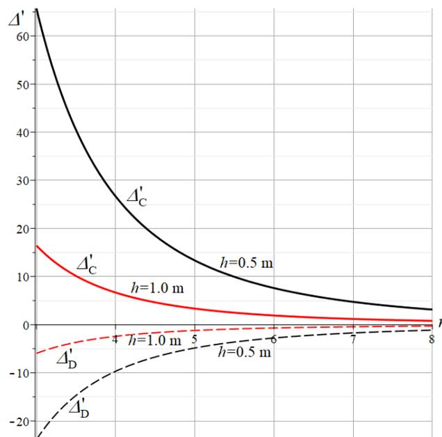
Fig. 4 - Relative deflections at points C and D at  $L = an = 40m$
