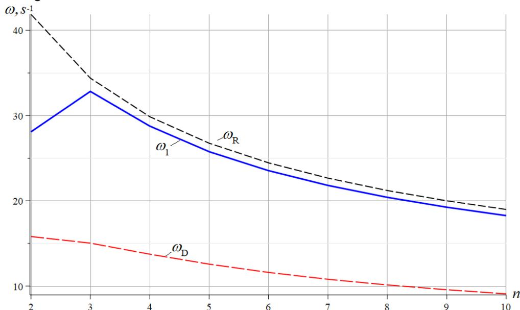
**Fig. 6 - Dependence on the number of panels of the first oscillation frequency  $\omega_R$  according to the Rayleigh method, the frequency  $\omega_D$  according to the Dunkerley method, and the first frequency  $\omega_1$  of the spectrum obtained numerically**
