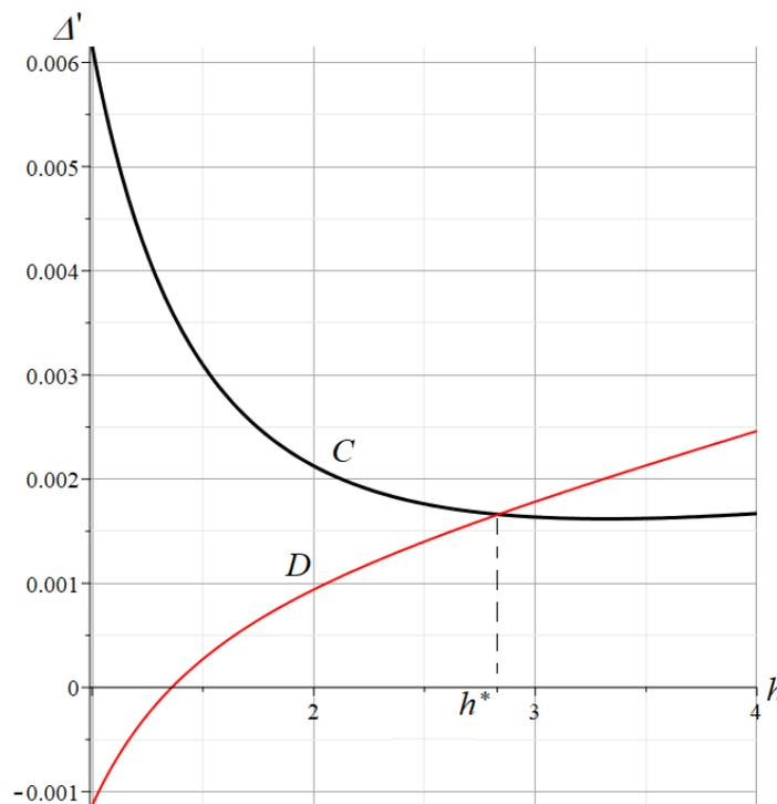
Fig. 5 - Relative deflections at points C and D at  $L = an = 40\text{m}$ ,  $n = 35$
