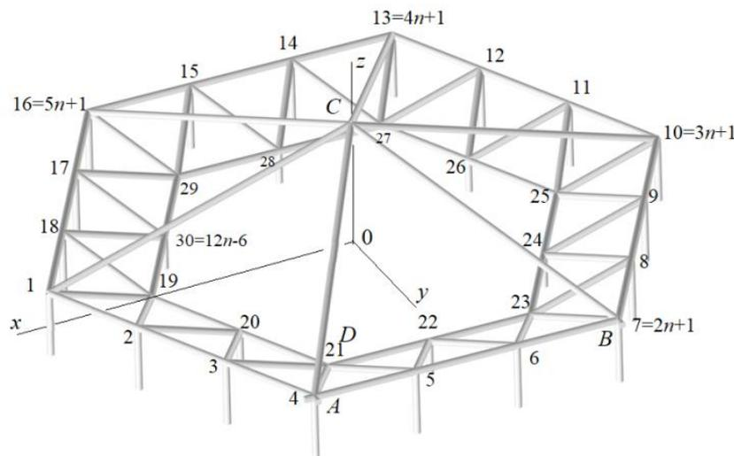
Fig. 2 - Truss node numbering,  $n=3$
