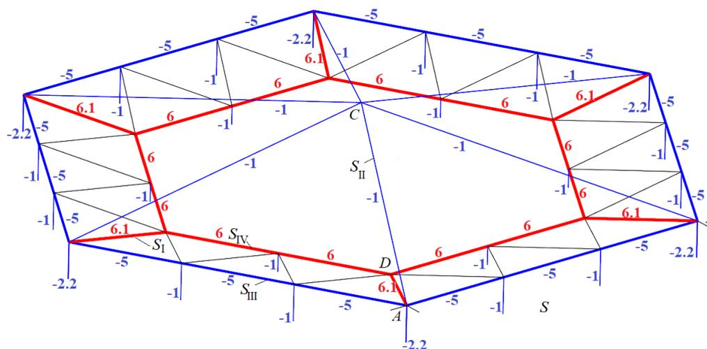
Fig. 3 - Distribution of forces in the truss rods,  $n=3$
