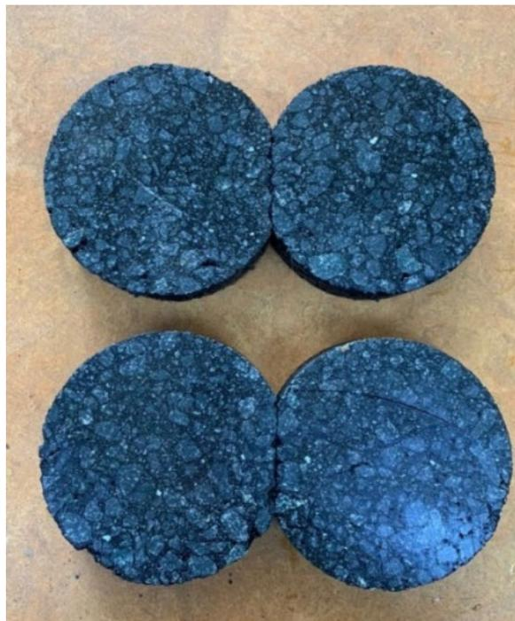
**Fig. 3 – Samples of asphalt concrete grade SP-16 in a cut.**
