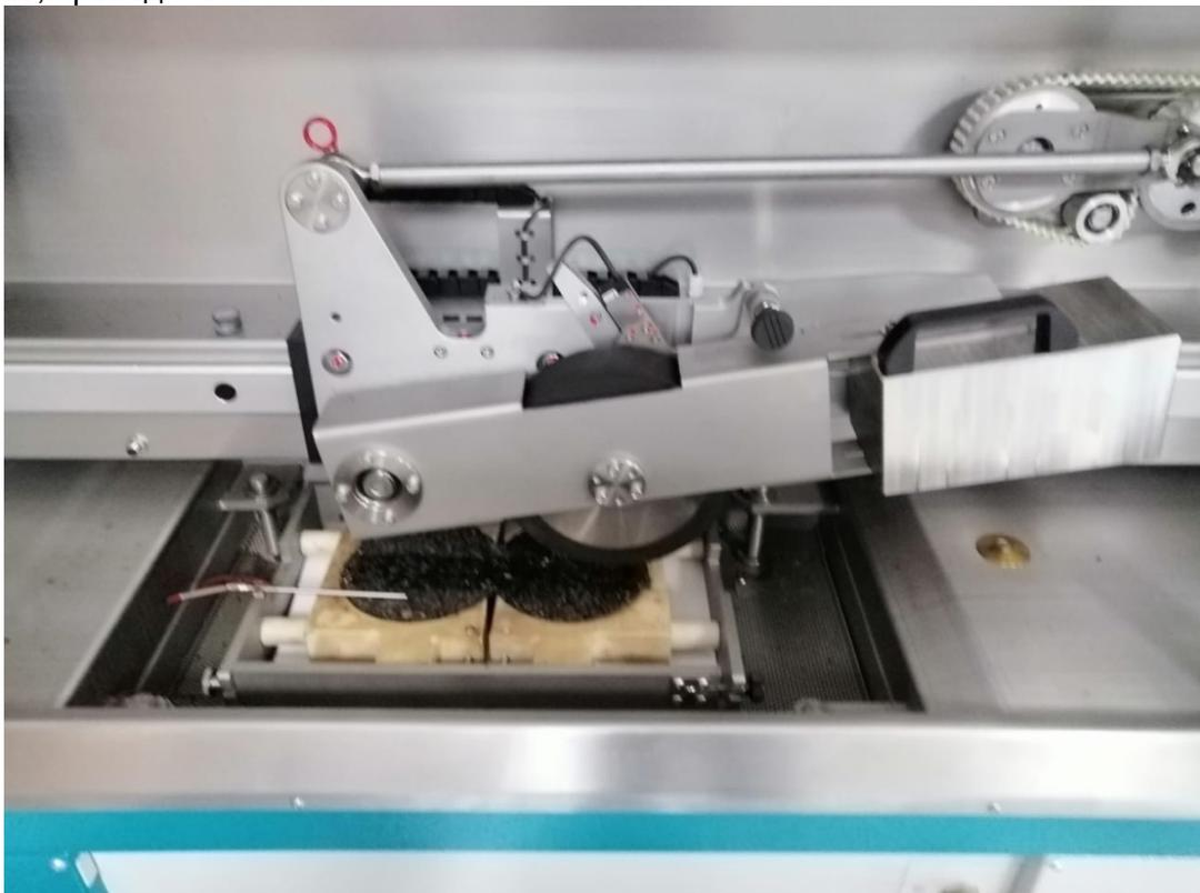
**Fig. 5 – Rutting Testing Machine with an Asphalt Concrete Sample Installed**
