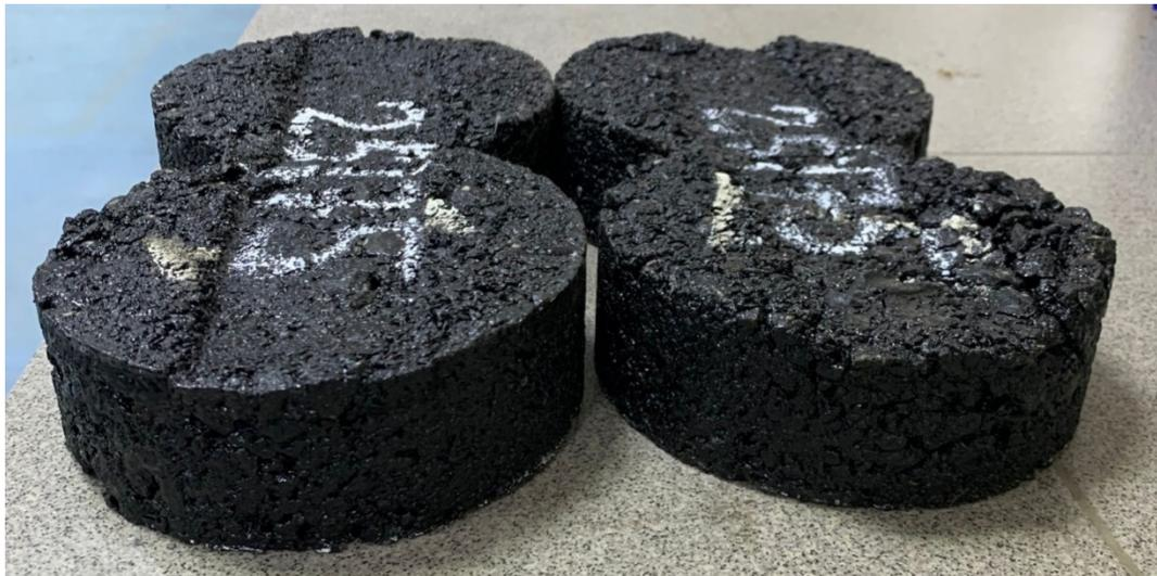
**Fig. 12 – Asphalt concrete samples SP-16 on BPV-25 bitumen after rutting test**
