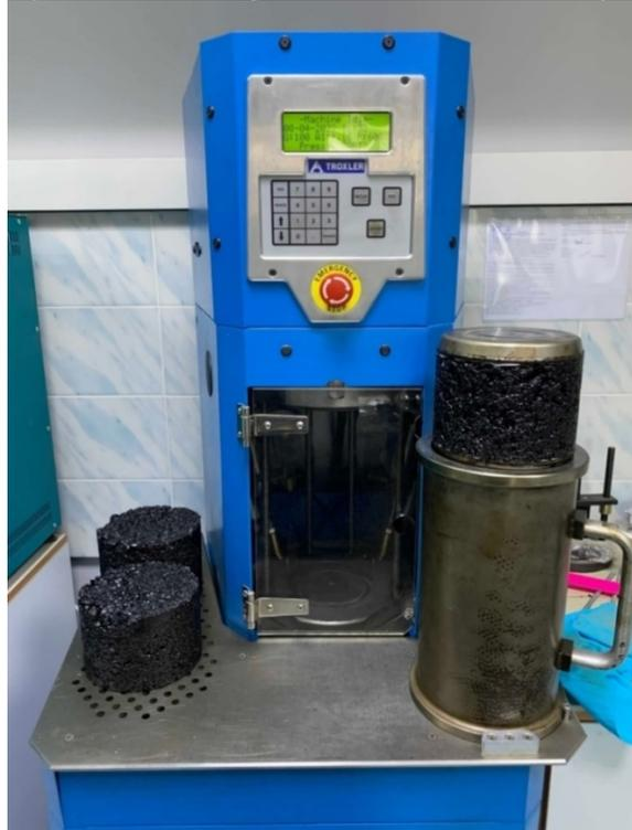
**Fig. 2 – Prepared samples of asphalt mix SP-16 on a gyratory compactor Troxler Super Pave Compactor 5850**
