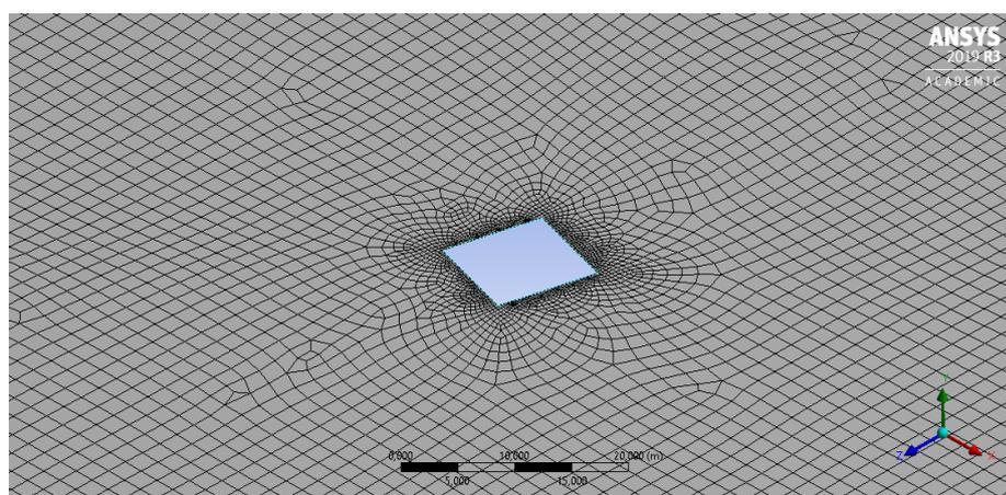
**Fig. 2 - Design scheme and its mesh in the Ansys SP**
