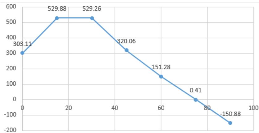
Fig. 9 - Graph of bending moment for the sides of the building with ratio of 1:4
