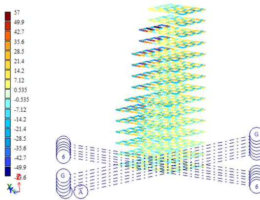
**Fig. 16 - Mosaic of bending moments in the horizontal plane in crossbars in the absence of a system of horizontal braces**
