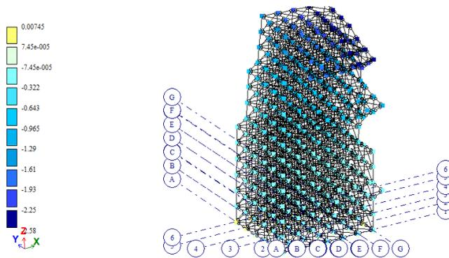
Fig. 14 - Mosaic of movements on Y without taking into account wind load unevenness
