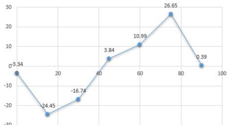
**Fig. 7 - Graph of bending moment for the sides of the building with ratio of 1:1**
