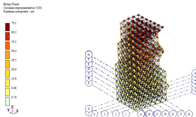
Fig. 15 - Mosaic of movements on Y taking into account wind load unevenness
