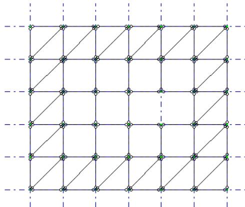
**Fig. 17 - Scheme of installation of horizontal braces**
