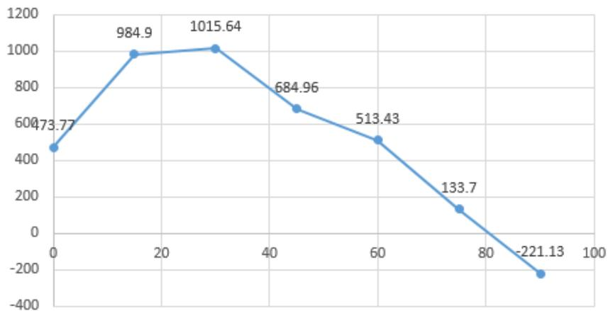
Fig. 10 - Graph of bending moment for the sides of the building with ratio of 1:6
