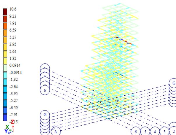
**Fig. 18 - Mosaic of bending moments in the horizontal plane in crossbars in a structure with a system of horizontal braces**
