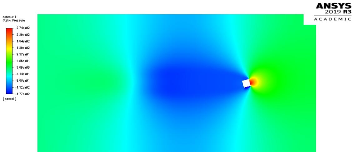
Fig. 4 - Static wind pressure around the design model
