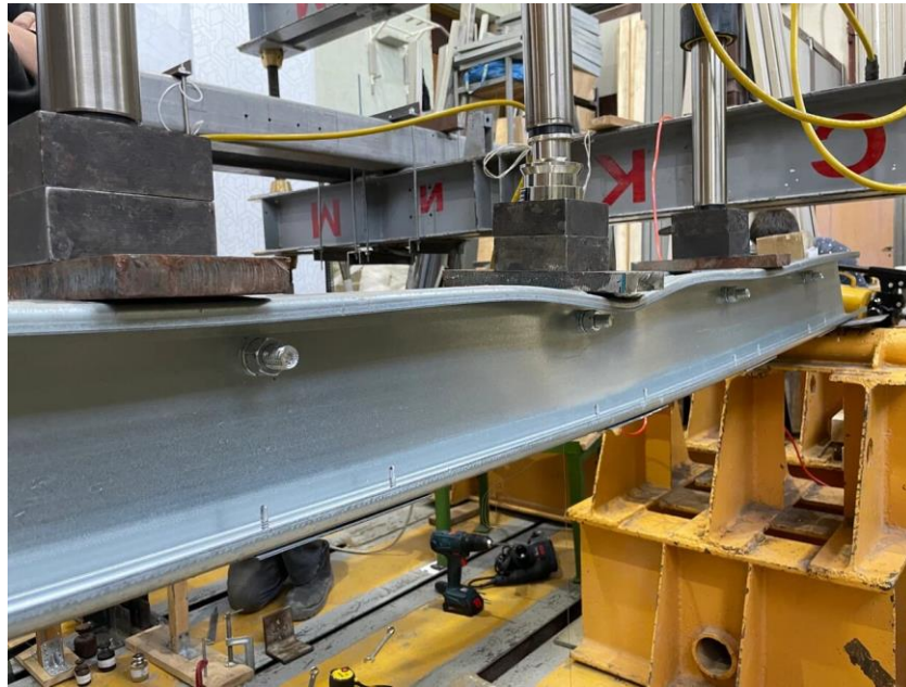
Fig. 9 - Loss of load-bearing capacity of the beam
