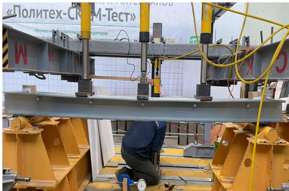
Fig. 8 - Testing of the beam sample
