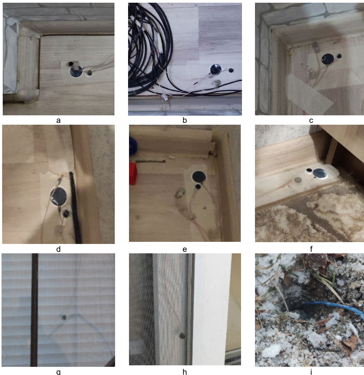
Fig. 3 – Location of temperature and surface heat flux density sensors in the room (a–f) and temperature sensors outside (g–i): a – point 1, module 559A; b – point 2, module 559A; c – point 3, module 559A; d – point 1, module 559D; e – point 2, module 559D; f – point 3, module 559D; g – point 7, module 559A; h – point 7, module 559D; and i – in ground
