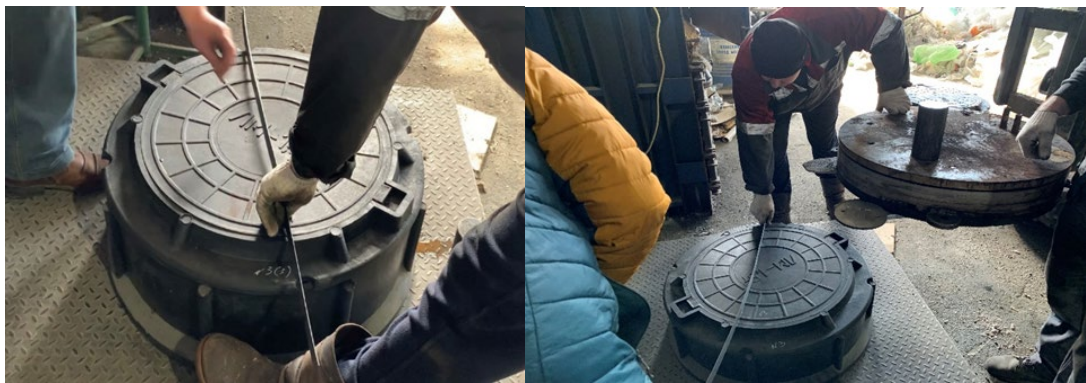
Fig. 1 – Experimental testing of manhole covers subjected to bending at a production site
