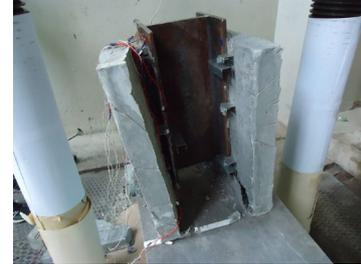
Fig. 3 Steel-reinforced concrete prisms in installation a) and after testing b)
