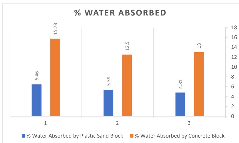
**Fig. 5 – Comparative Analysis of Water Absorption Test**
