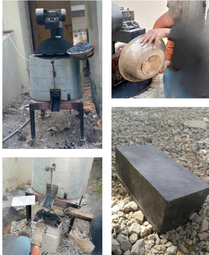
**Fig. 3 – Production Procedure of ABS Plastic-Sand Composite Bricks**
