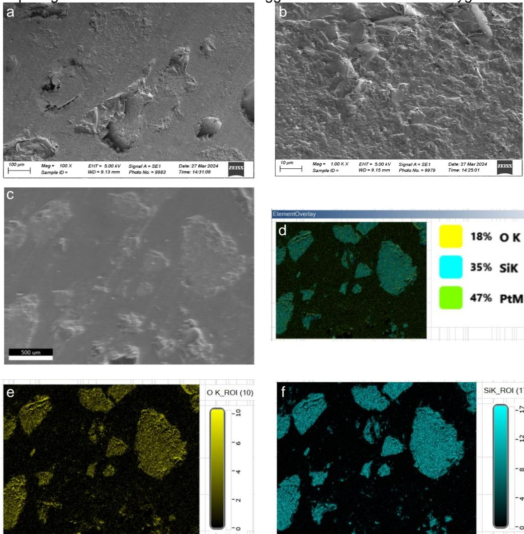
**Figure 7 – The SEM micrographs and energy dispersive spectroscopy (EDS) maps of produced plastic sand composite block: (a) SEM micrographs at 100X; (b) SEM micrograph at 1,000X; (c) SEM-EDX map location; (d) overlay of elements in EDS map; and corresponding mapping images of oxygen and silicon, (e) and (f), respectively**
