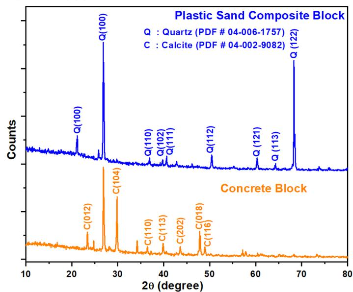
Figure 6 – X-Ray diffractograms of concrete block and plastic sand composite block
