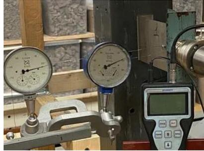
Fig. 9 - Compression testing stand
