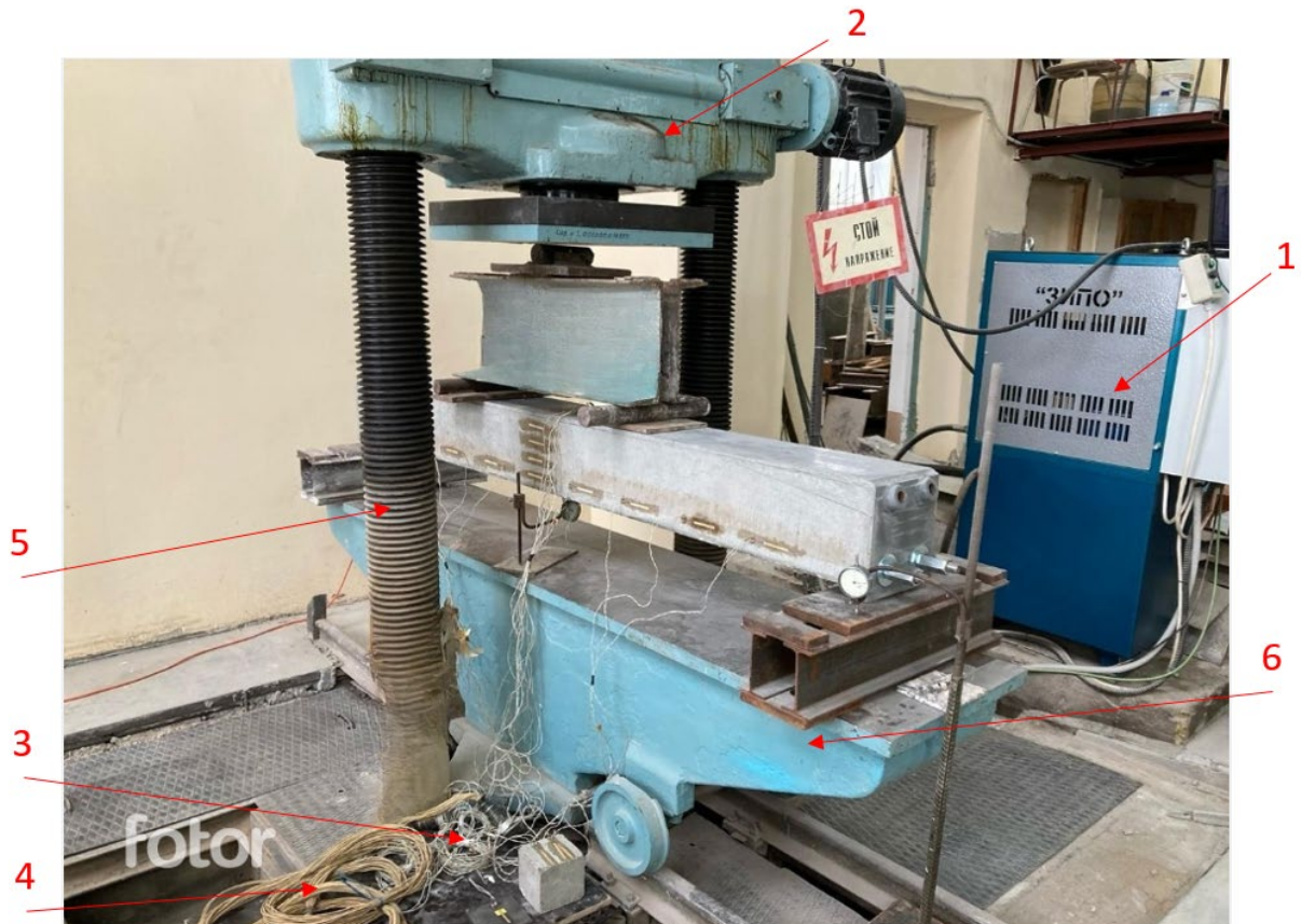
Fig. 4 - Schematic diagram of the test setup: 1 — loading unit of the press; 2 — fixed support; 3 — signal switchboard; 4 — cable; 5 — press columns; 6 — press base Image by the author of the article
