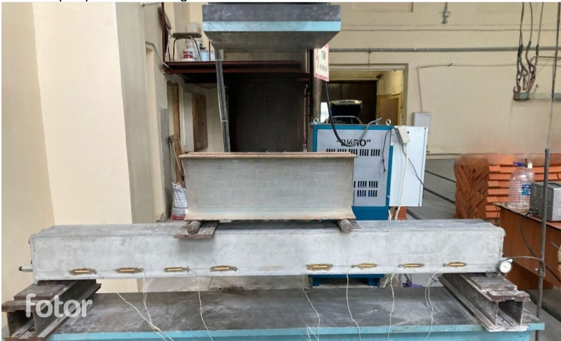
Fig. 3 - General view of the beam installed on the test stand
