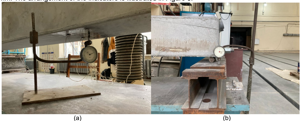
Fig. 5 - Arrangement of dial indicators: (a) mid-span deflection measurement, (b) support settlement measurement Image by the author of the article
