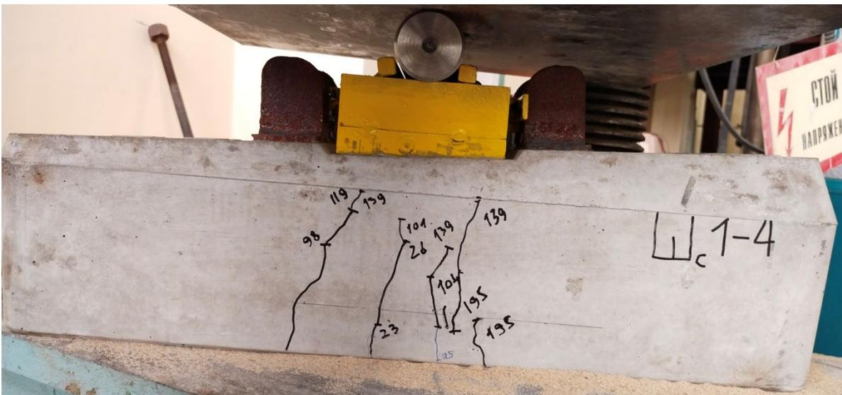
Fig. 4 - Sample of a half-scale during loading, formation of inclined cracks
