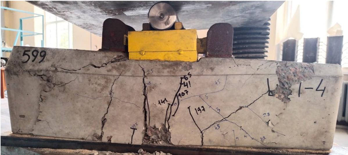
**Fig. 5 - The moment of failure (destruction) of a half-sleeper**
