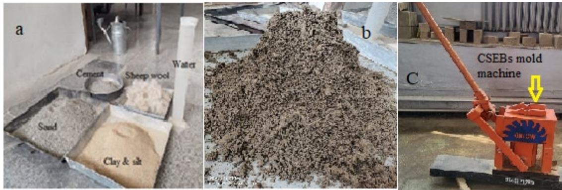
Fig. 1 - Show: a) CSEB raw materials, b) mixture for CSEBs, and c) CSEBs production molding machine
