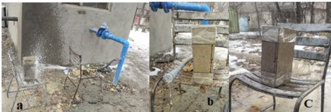
Fig. 8- Show results of the water erosion test on CSEBs: a) brick during the experimental condition; b & c) CSEBs after the test, showing no erosion observed
