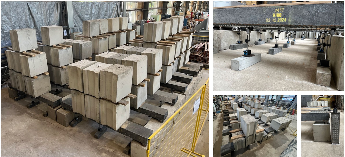
Fig. 4 - Long-term testing of samples of beams by gravity load Image by the author of the article
