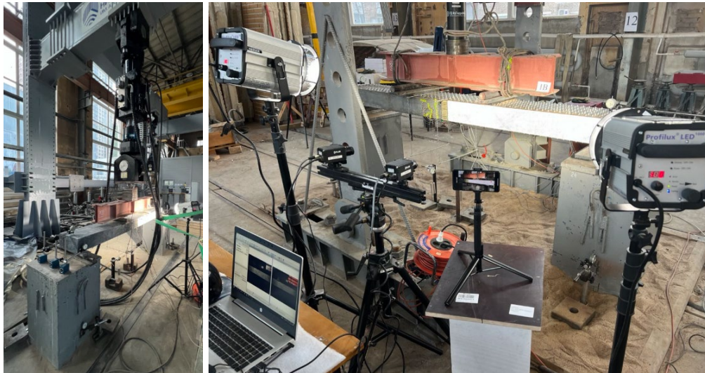
Fig. 2 - The testing process and operation of the VIC 3D system for monitoring the cracking process in the beam
