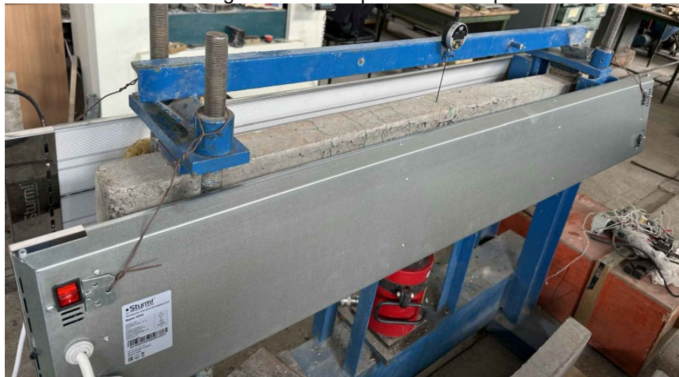
Fig. 7 - Heating with infrared heaters
