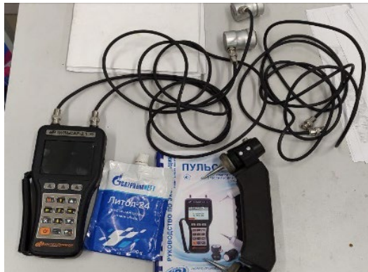
Fig. 3 – Ultrasonic device PULSAR-2.1 [13]
