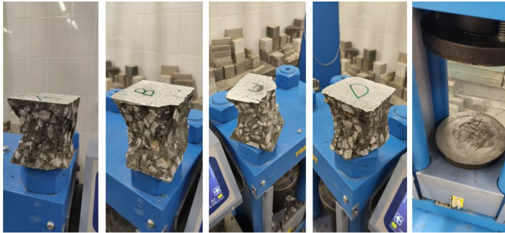
Fig. 13 – Concrete specimens after testing on the C040PN machine
