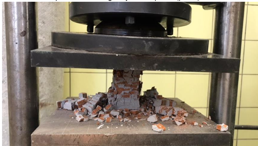
Picture 7. Tests of brick columns of automated assembly after damage
