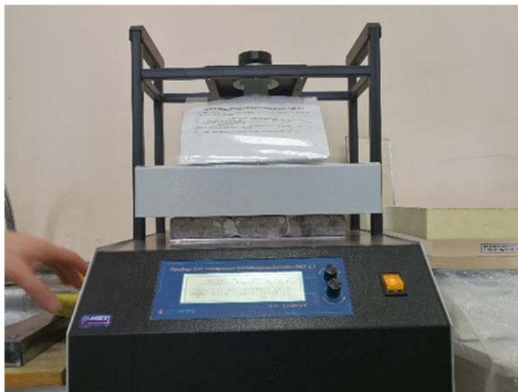
Fig. 5. Thermal conductivity test of expanded clay mixture plate
