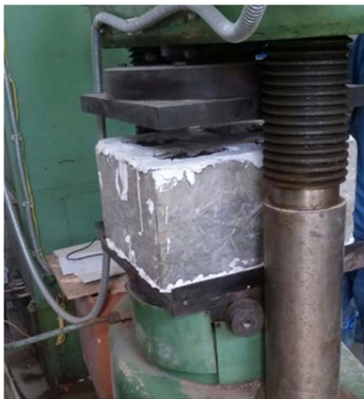
Pic. 4. Leveled block under the press
