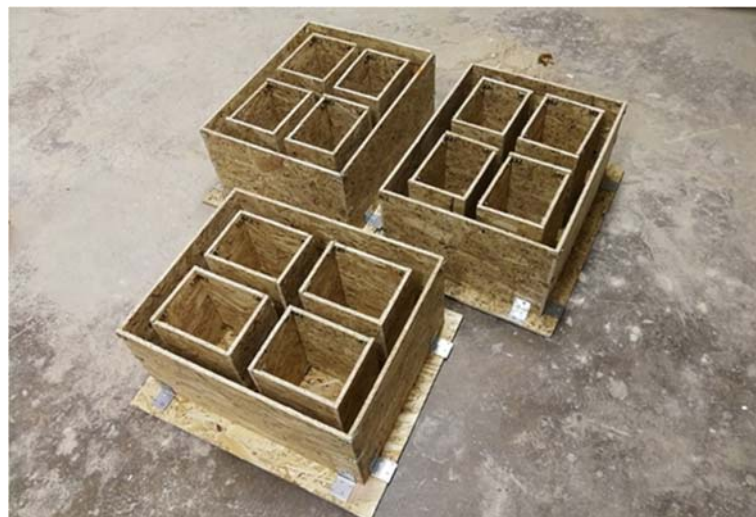
Pic.2. Formworks for designed blocks
